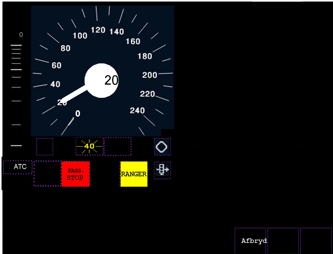
Passage Stop during Shunting 5__ AWAITs PASSAGE OF NEXT STOP-SENDING BALISE Yellow display flashes
